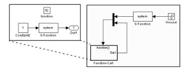
Such models cannot be correctly simulated. Accordingly, Simulink software now displays an error message when you attempt to run or update a diagram containing function-call cycles.
