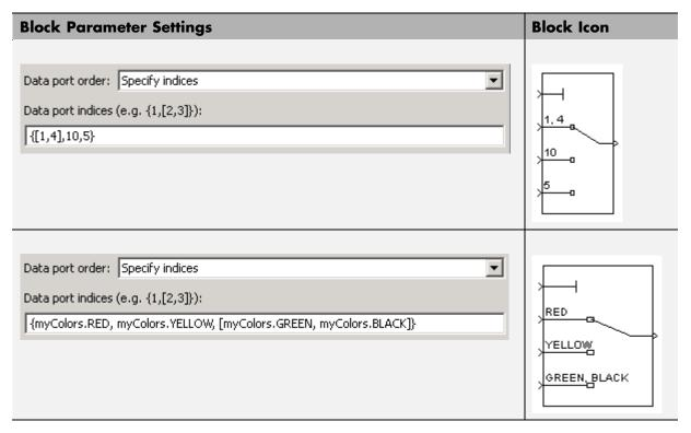
When you load existing models that contain the Multiport Switch block, the following parameter mapping occurs:
